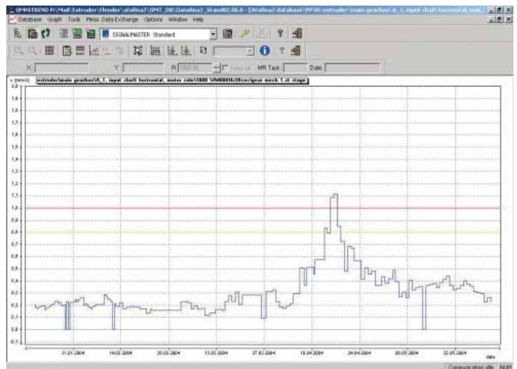
Figure 4: Trend progression with a brief rise in amplitudes of the gear mesh frequency of the drive stage. The rise was automatically transmitted by eMail.
