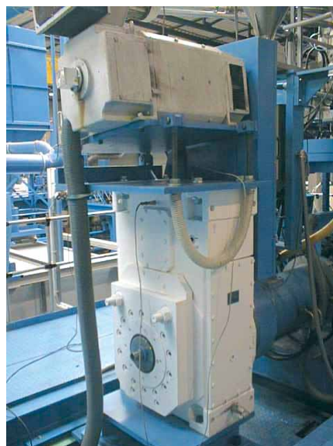
Figure 2: Drive configuration of damaged single-screw extruder
