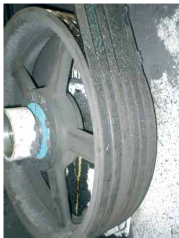
Figure 1: Belt drive of single-screw extruder after removal of protective enclosure
