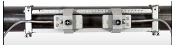
Measurement with transducers mounted with the portable Variofix VP
